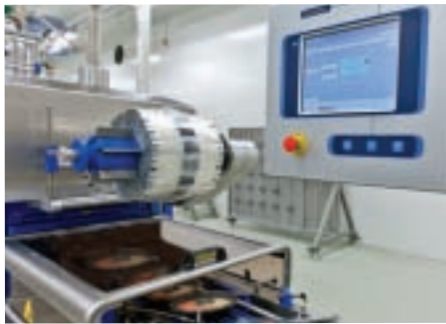
A special valve is applied to the top film
