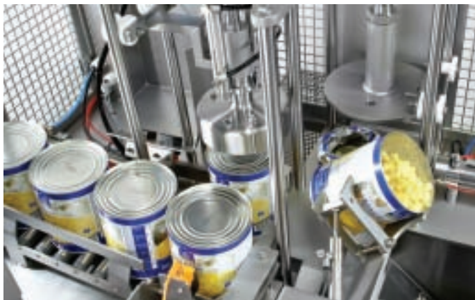
The tilting operation combines with compressed air and a water blast process to ensure all contents are removed from the cans
