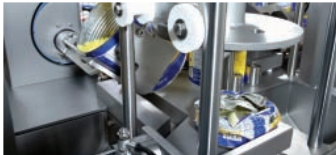
Empty cans are transferred to a can compression facility before being ejected from the unit for disposal off-site
