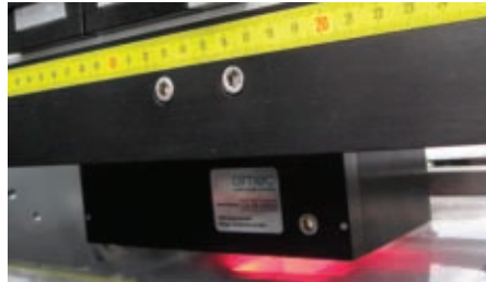
Olmec's seal inspection system ensures the integrity of four sided seals for dressings
