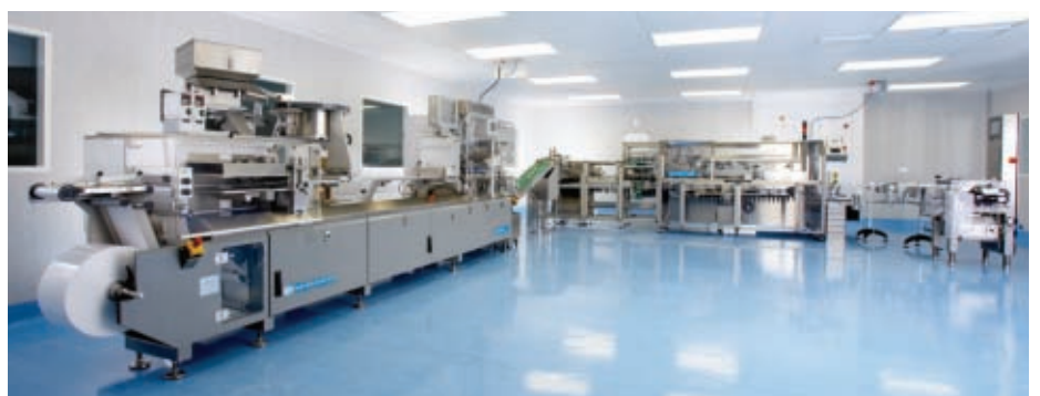
The Hay-on-Wye sites houses a Noack 623 blister packer and Promatic PC 4200 cartoner
