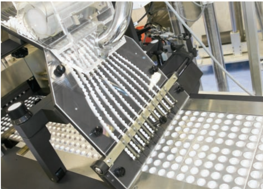
Dedicated feeders are used for difficult to handle or fragile products at Brecon
