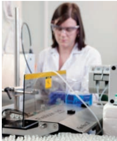
The FF20 is a filling system for medium sized runs of up to 2000 units an hour
