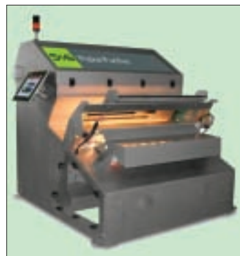
The 2500 S+S flake purifier SM300 sorts mixed plastics flakes
