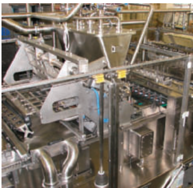
The Waldner Dosomat 20.8 showing the packaging cleansing area, main filler and sterile air tunnel
