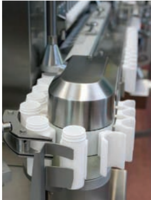
The MT1000 rigid tube filler
