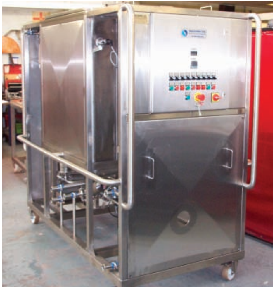
CIP where it's needed: Typical mobile Suncombe CIP unit can be moved from line to line
