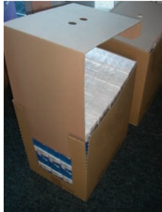
Side-loaded case: Tissue packs are loaded into this two-piece case on a Focke machine
