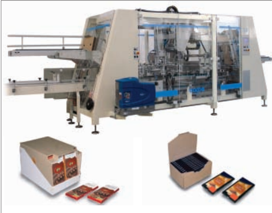
Wraparound or two-piece display: Cama FW 749 Combi case packer can produce both styles
