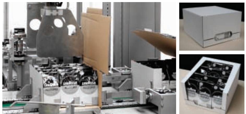
Choice of pack style: MAF Combimatic shown creating a wraparound solution using a perforated blank
