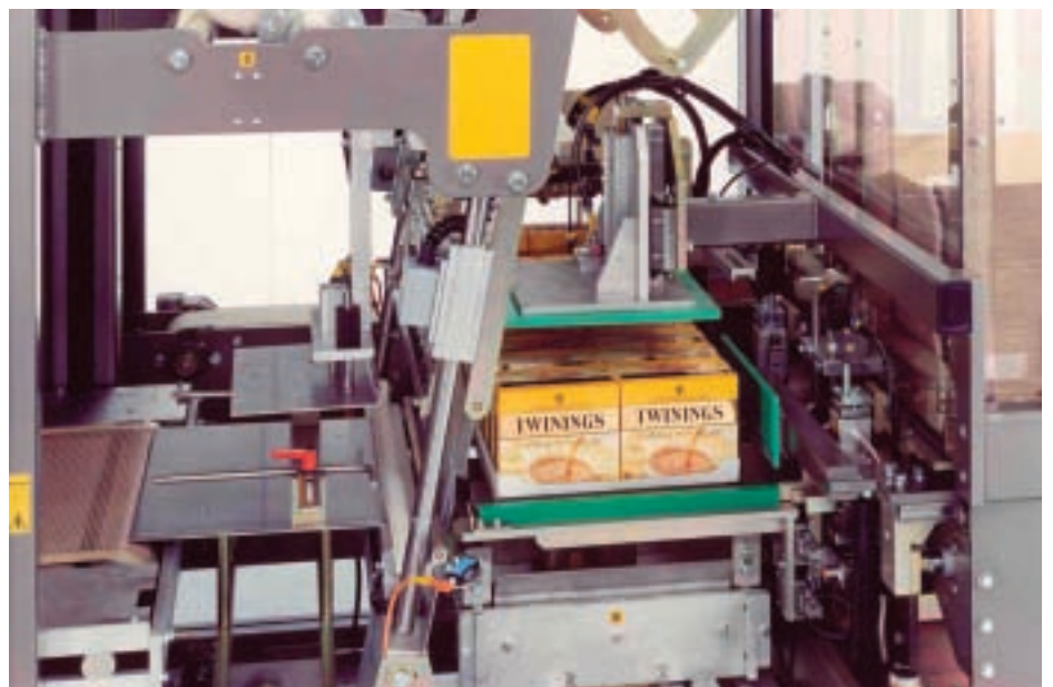
Three operations in one: Europack shrink/tray wrappers have been installed at Twinings, Tyneside
