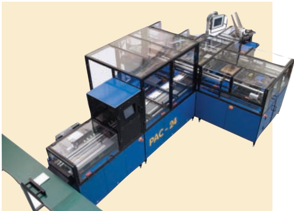
Applying stamps: PAC-24 machine uses Festo drives to provide high accuracy positioning
