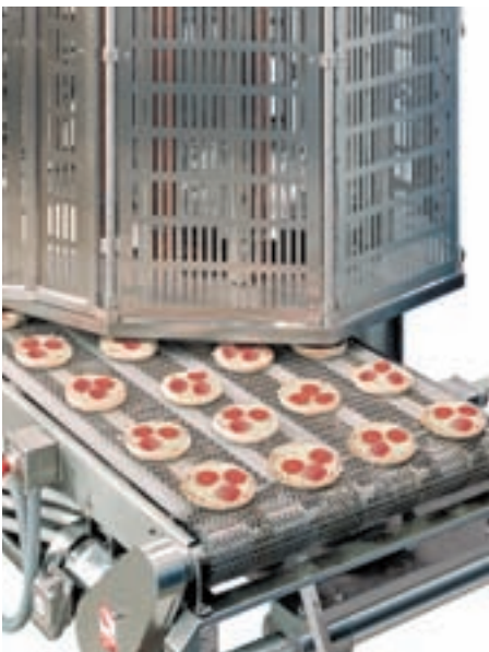
Cut and place: Pizzamatic machine supplied by JBS slices and places product such as pepperoni
