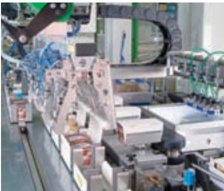
Yogurt pots: Multipack assortments are created and loaded into board sleeves by this line
