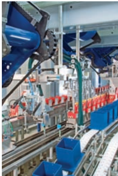
Tea bag cartoning: Product is loaded into the blue carriers and then tipped into the cartons
