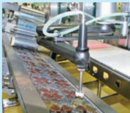
Continuous motion: The thermoforming lines are fed by robot from the central product infeed
