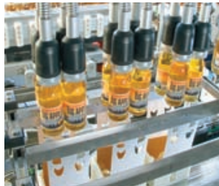
Bottles: One of several machines for loading bottles into board multipacks, erected and carried in pucks
