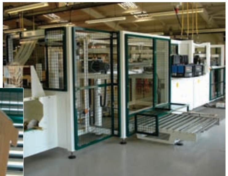
Servo driven: The Europack machine (above) secures film to board to create the Smart Karton transit case blank (left)
