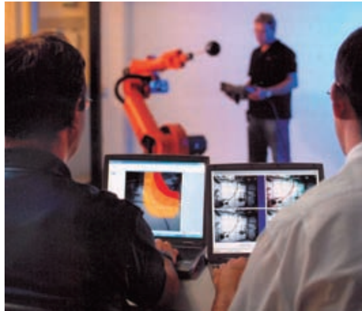
Camera-based safety: New Pilz SafetyEye gives three-dimensional zone monitoring
