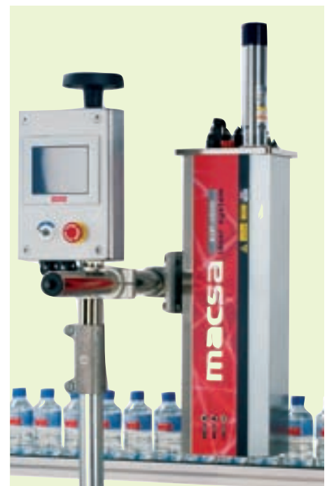
Faster coding: Macsa K-1000 SHS is capable of speeds up to 500 metres a minute
