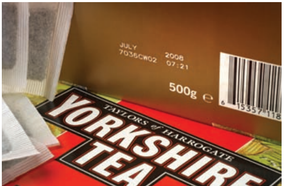
Multi-lingual codes: Taylors of Harrogate is using scribing lasers from Linx to code its tea cartons
