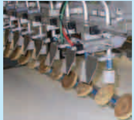
Stacking the inverted tier: The row is lifted, turned over, and then picked again for transfer face down
