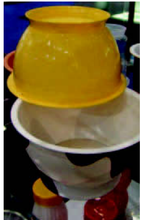
Pedestal pots: Made on the Erca-Formseal system
