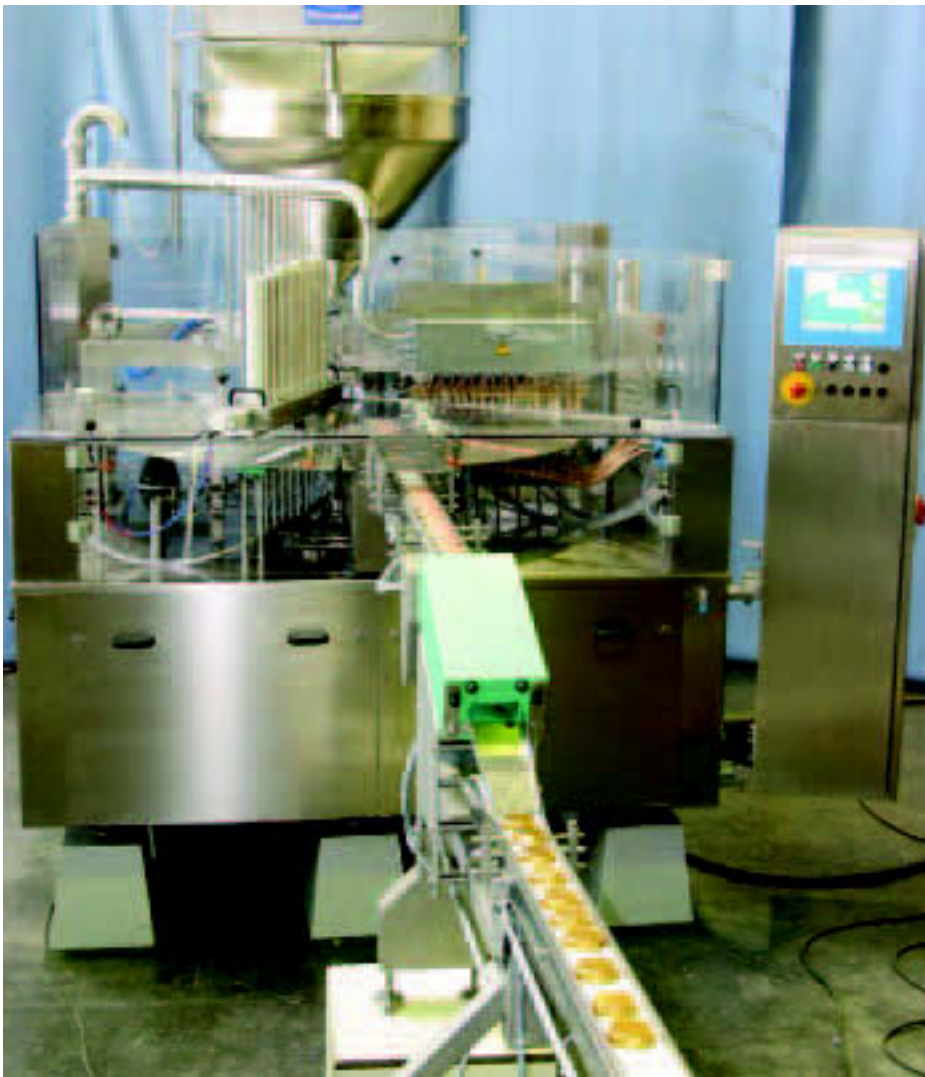
Multilane rotary: Waldner rotary eight-lane machine for filling and lidding aluminium cups
