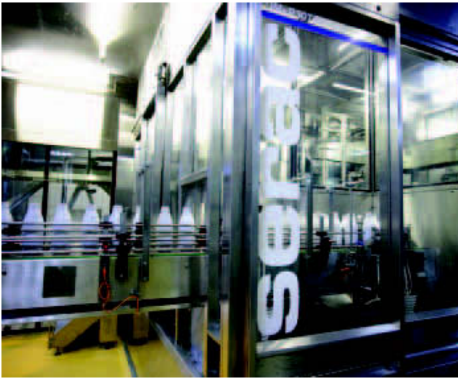
RABS for aseptic filling: Above: Serac has applied pharmaceutical industry RABS technology to the drinks industry, offering 72 hours continuous production with no need for intermediate decontamination. Below: The concept: 1: Sterile area. 2: Barrier zones. 3: Glove boxes for access to sterile area during operation
