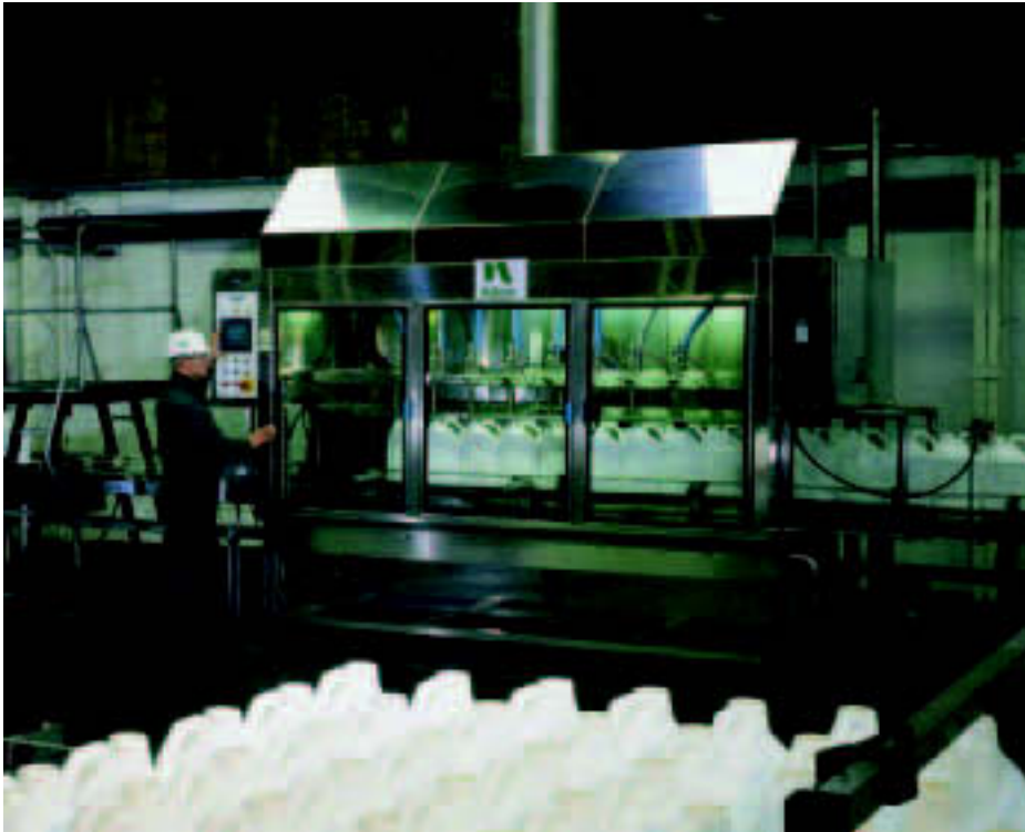
Flowmeter filling: The heart of the new Nufarm line is an eight-head Masterfil machine
