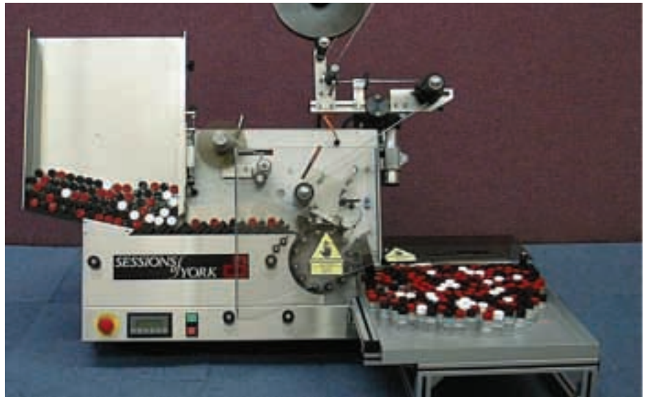
Labelling cylindrical items: Sessions' RC30 uses a walking beam for indexing the containers
