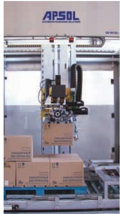
Pick-and-place: CP-G Robot from Italian manufacturer Apsol can lift 40kg
