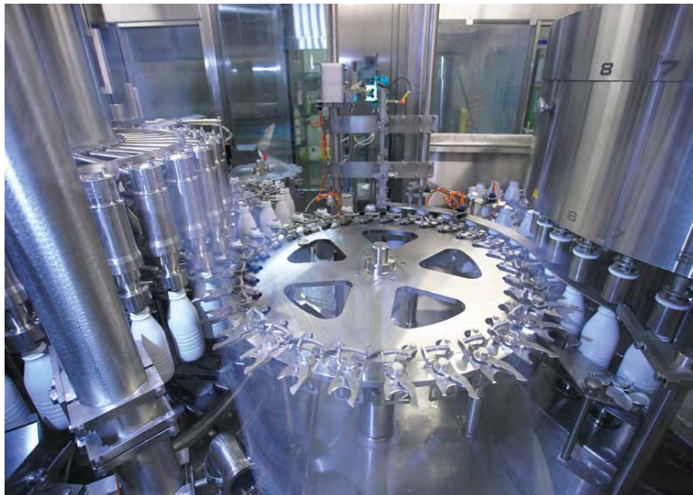
Serac aseptic filler: Much R&D effort has gone into handling sports cap sterilisation
