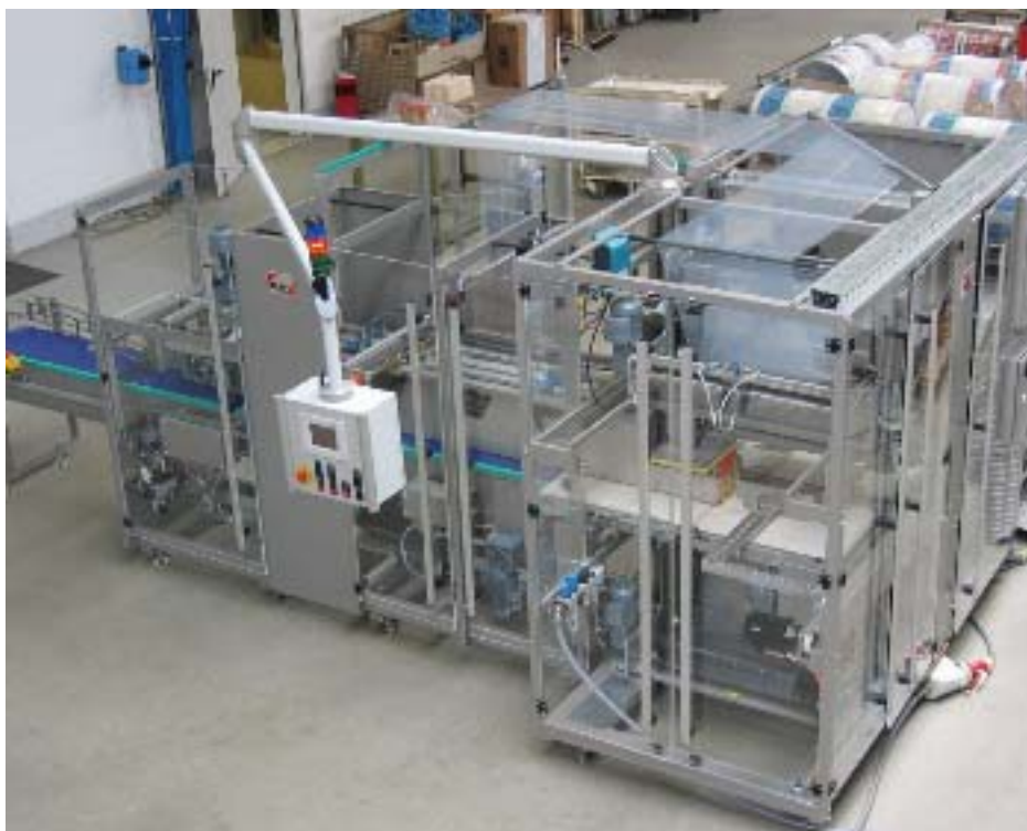
Servo drives: MAF Servo Fox stretch-shrinkwrapper gives speeds up to 50 cycles a minute
