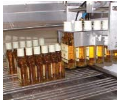
Unsupported bottles: Polypack machine is loaded with a pick-and-place device
