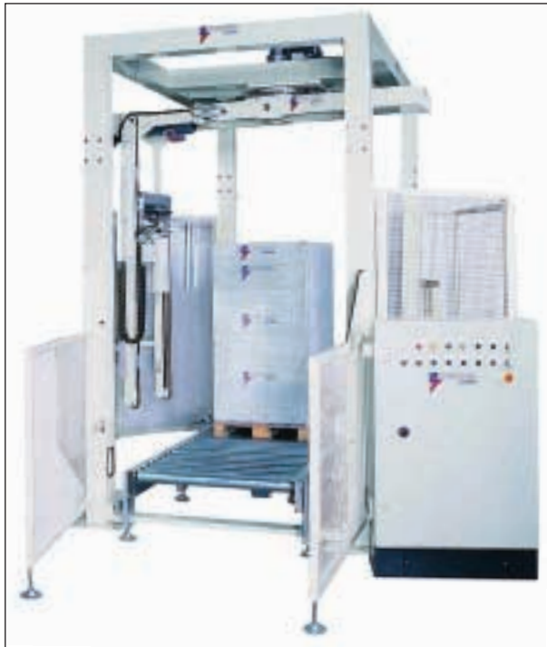
Robopac wrappers: Above: Helix HS40 rotary arm machine as supplied to Silver Spring. Right: Office furniture is also protected by stretch wrapping
