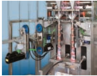
Twin tube bagger: ContiBag 40/26 duplex
