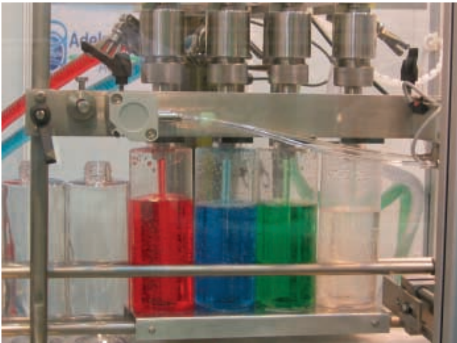
Choice of format: Adelphi Response Automation System filling four different liquids into different bottles
