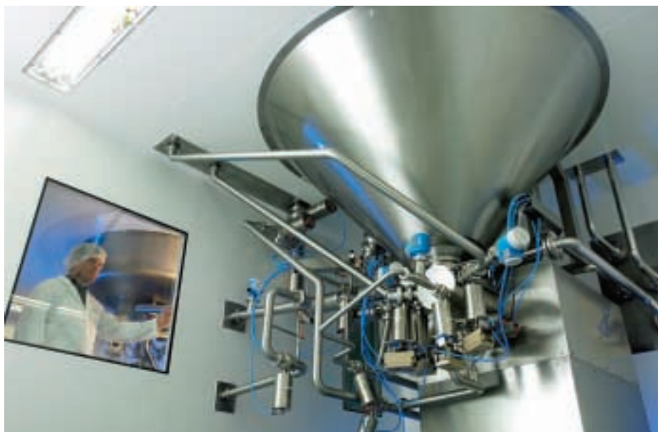
One step processing: FrymaKoruma Dinex 5200 installed at contract packer ASM in Switzerland
