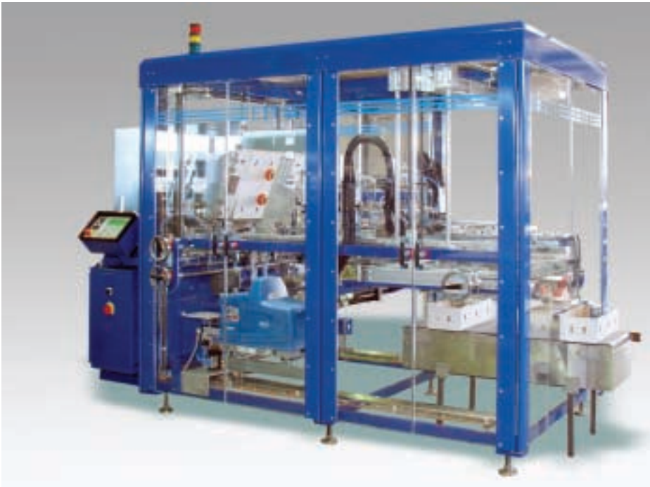
Shelf-ready tray loader: ETT TFS40 machine from Engsol handles "tottles" at 150 a minute
