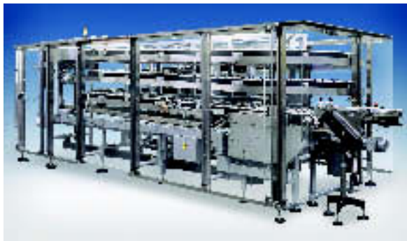
SIG pack buffer: Inclined chain with pockets for the product creates a 'multi-storey car park' effect
