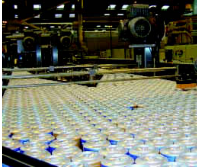
Improved handling: New Dawson matt top can conveyor at Barr Soft Drinks
