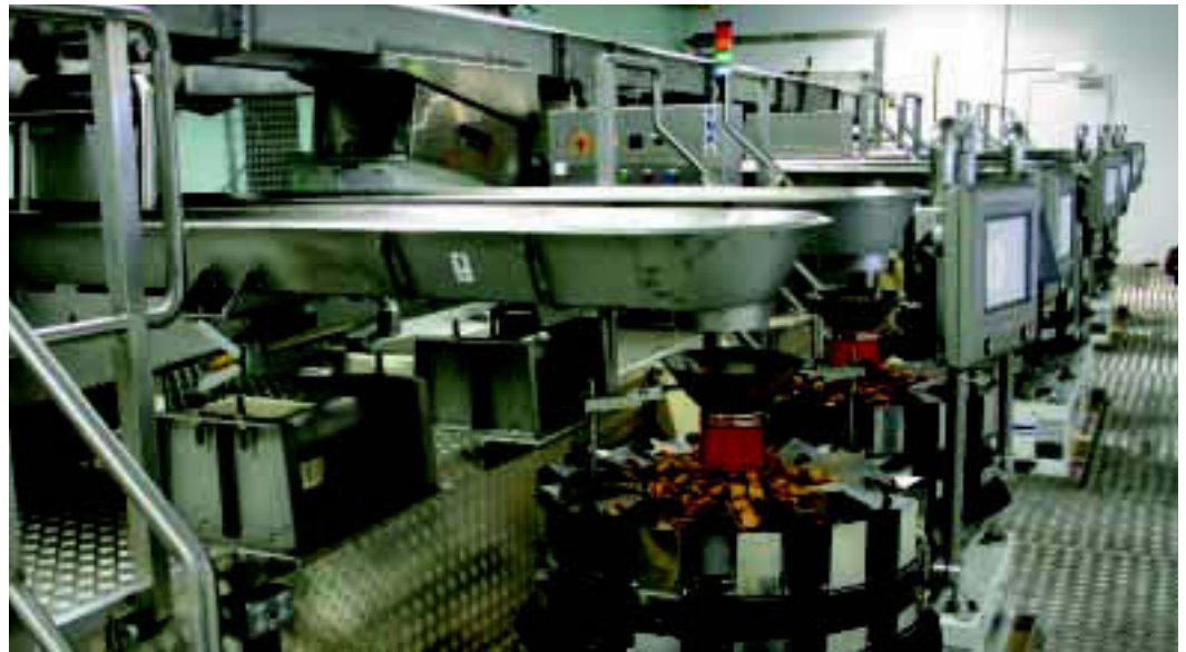
Servo controlled: TNA Roflo distribution system employs horizontal motion conveyors
