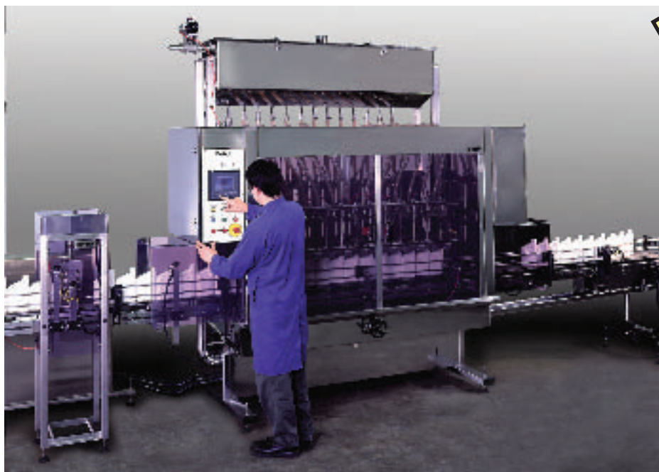
Automatic line: Masterfil 12-head filler has substantially reduced changeover times
