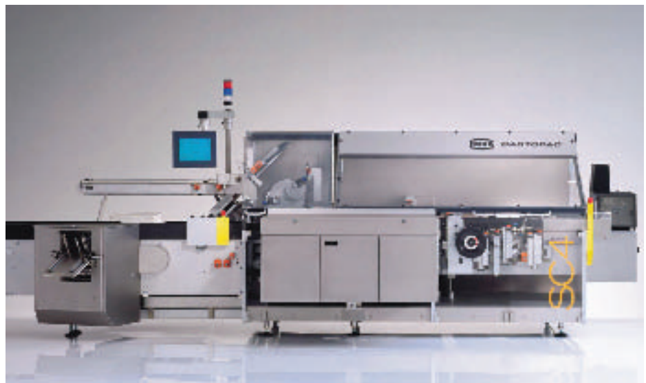
Continuous motion cartoner: IWK Cartopac SC4 gives speeds up to 450 cartons a minute
