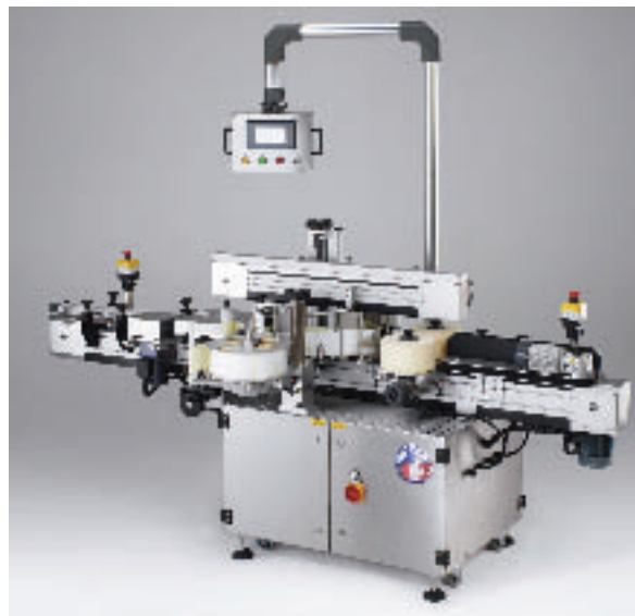
Front and back labeller: Pals 70FBL machine now has a colour touch screen control
