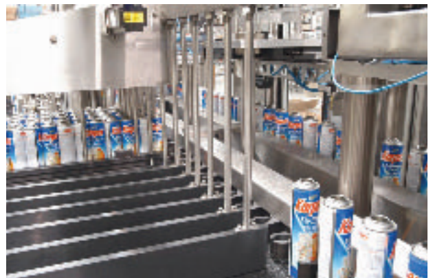
Servopak filler: Uses peristaltic and gear pumps for quick changeover
