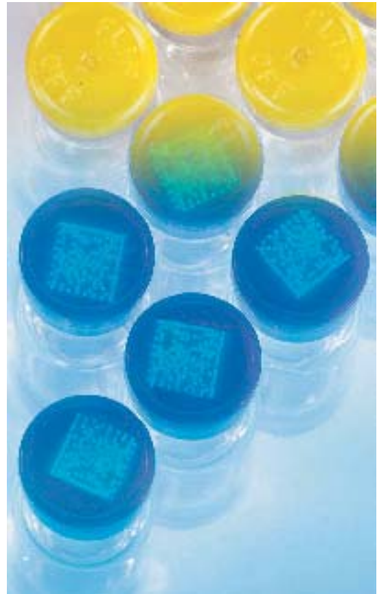
Coding vials: Searle is using ultra-violet inks and a Domino ink jet to apply data matrix codes
