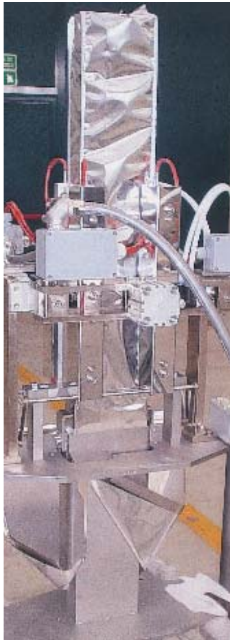
Four corner seal: Ricciarelli forming tube has built-in sealing elements for fast changeover
