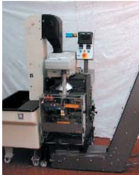
Bullion bagging: Complete system from GIC with bulk feed elevator and bag counter
