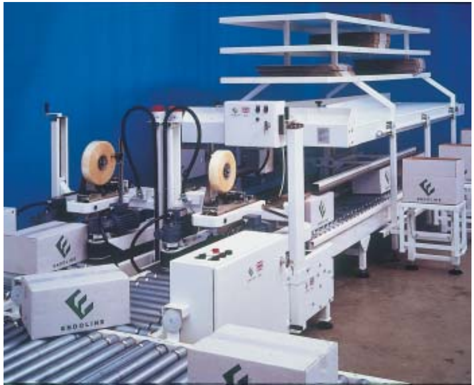
Hand packing station: Ergonomic system from Endoline feeds into automatic case-taping machines
