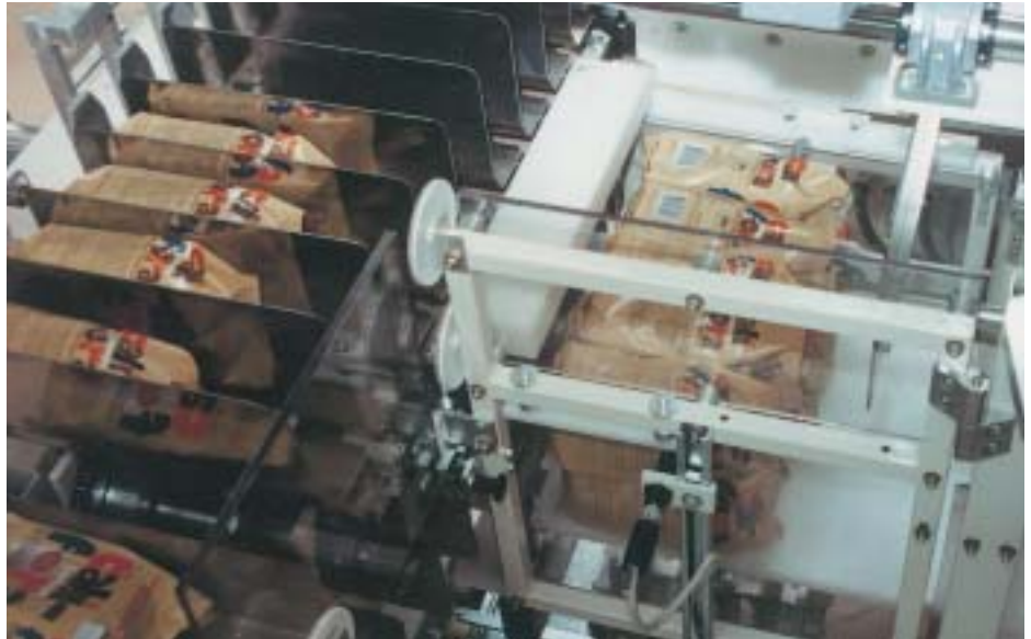
Handling flexible packs: Cermex racetrack collator presents bags on edge for side-loading into cases
