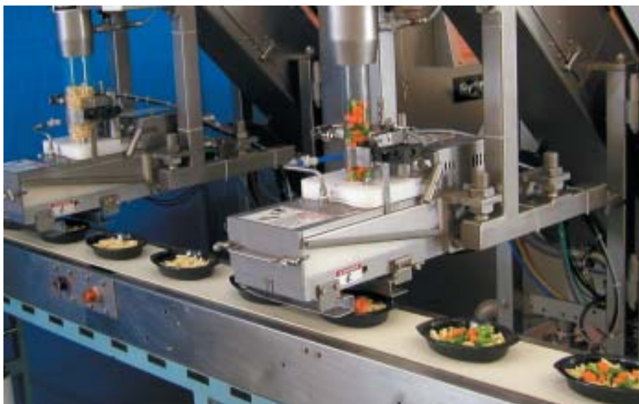
Pasta with two veg: Multi-Fill MPF is said to deliver difficult products accurately
