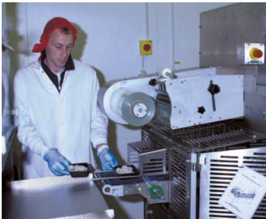
Automation: Tray sealing on one of the two Packaging Automation Vision 182 machines
