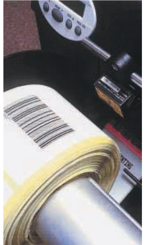
Bolt-on scanner: Veriscan from Sessions checks legibility of bar code print
