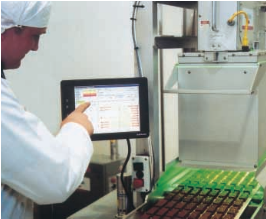
Monitoring coating weight: The Dipix 3D vision system has been introduced by APV Baker
