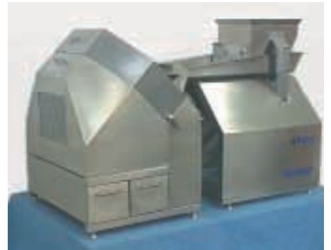
Bolt-on scanner: Veriscan from Sessions checks legibility of bar code print
