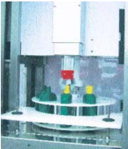
Rubber fingers: The Cap Coder CC550 starwheel-based capping machine
