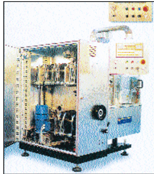
Easy access: Puma 100 tube filler from Packaging & Design has drive elements arranged vertically
