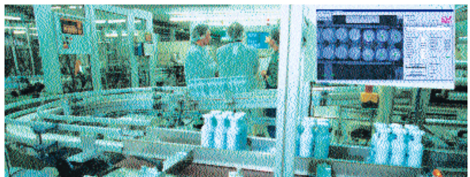
Transit pack inspection: At the second station, the system monitors bottles in six or 12-packs
