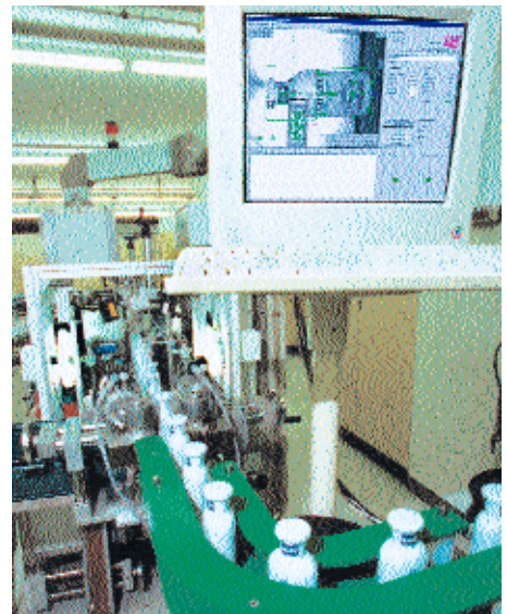
Front, back and cap: Station one inspects both the labels and the closure
