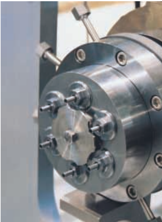
Half as much again: Output of filled snacks can be raised 50 per cent with APV Baker's six-stream die
