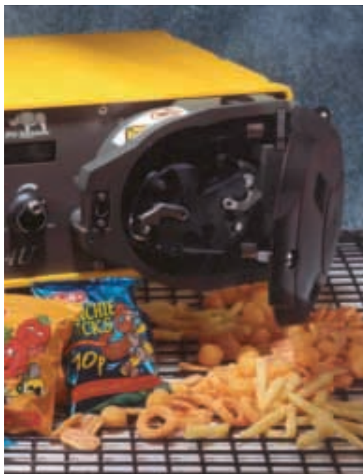
Metering flavours: Watson-Marlow Bredel peristaltic pumps have been adopted by Red Mill
