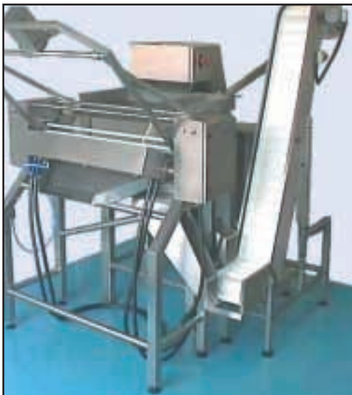
Sorting lightweight products: Radix AS322 machine occupies only 1400mm of line space
