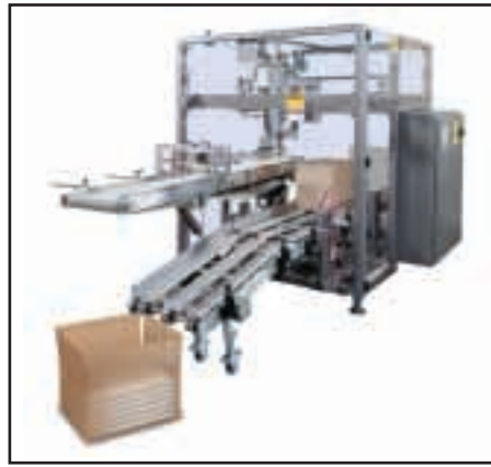
Pick-and-place: MTL100 machine from US manufacturer SWF for handling flexible packs
