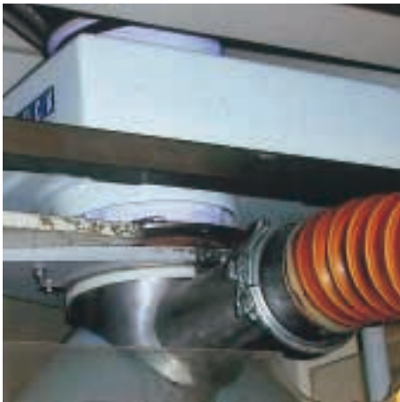
Throat detector: Lock's new Waferthin model is 25 per cent smaller than previous units
