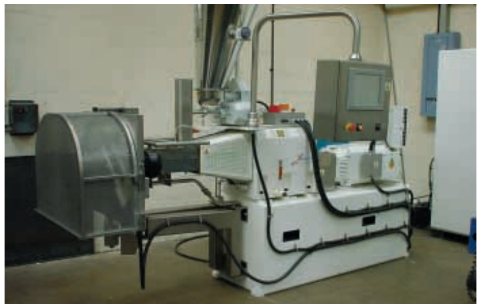
Simple concept: ABT twin screw extruder from Planet Flowline for expanded snack food lines
