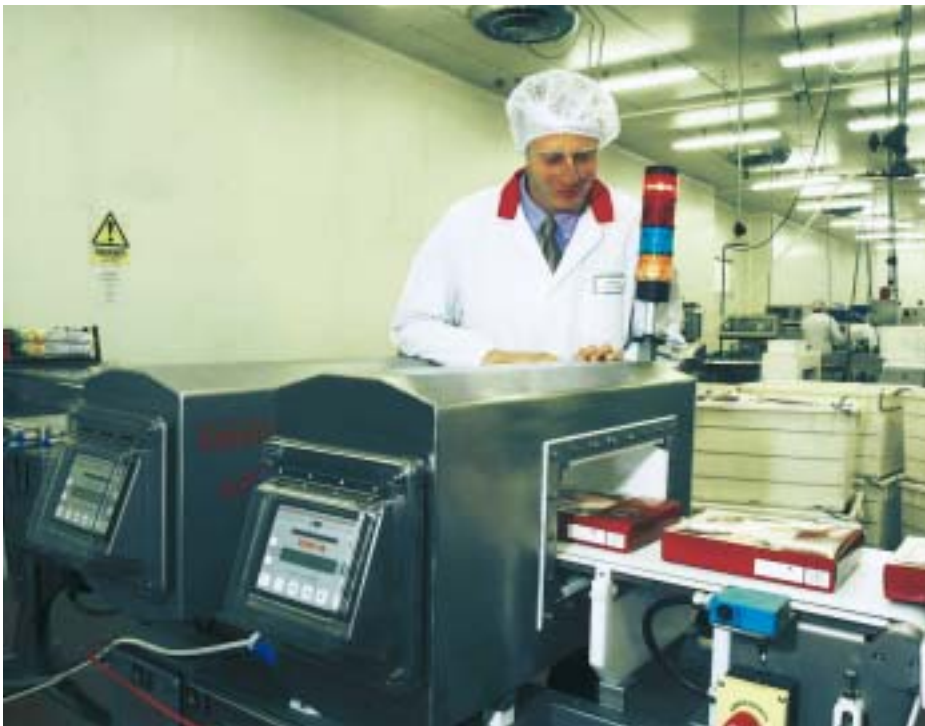
Twin heads: Evesham Foods is using a two-bead metal detector from Safeline
