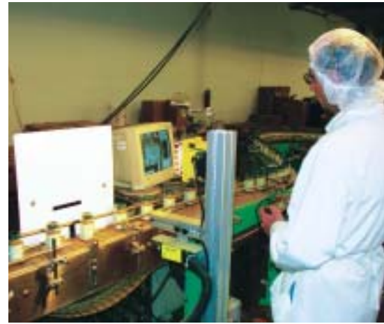
Inspecting spice jars: The Cognex system in operation at US packer Spice Hunter
