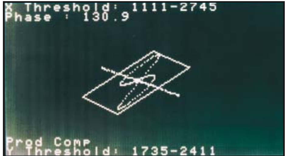
Sensitivity in sight: Willett MD7600 shows product effect within a box that can be tightened or loosened
