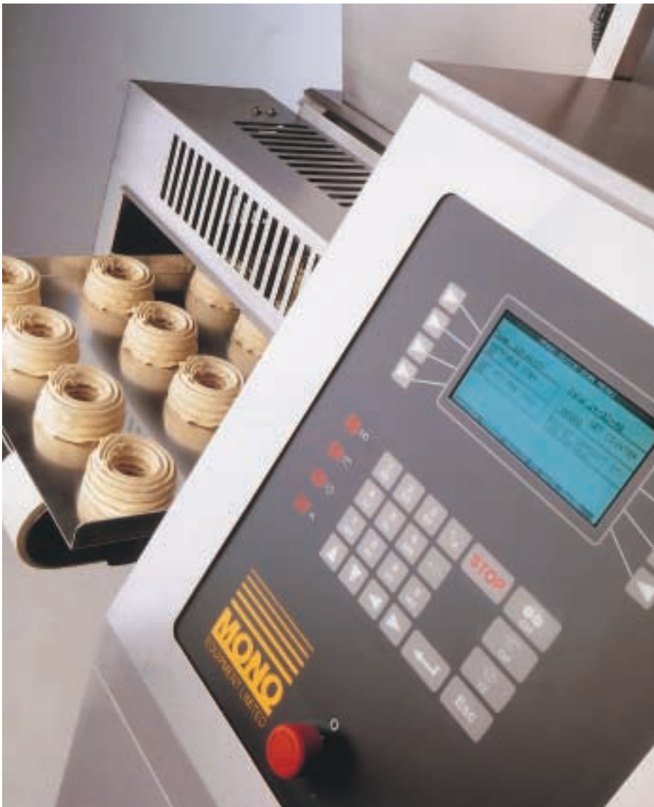
Mass customisation: Mono Equipment's Delta confectionery depositor takes on the work of skilled hands
