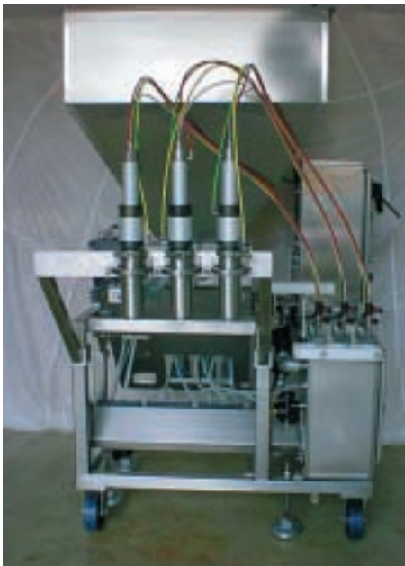
Three heads: Paletborpes is using a new Raque PF-2.5-3 filler for pie fillings
