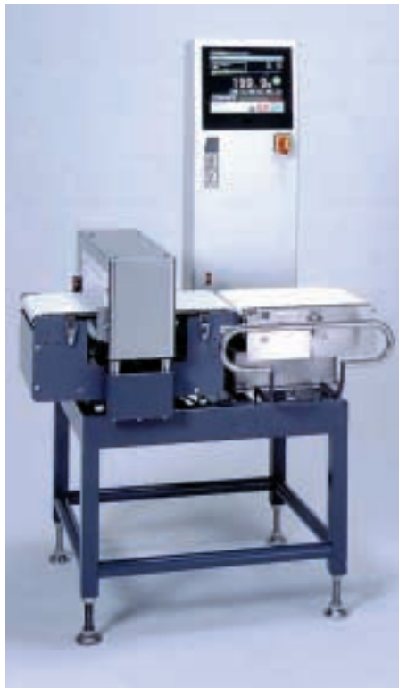
High Speed: Anritsu SV series checkweigher with metal detector on a common frame
