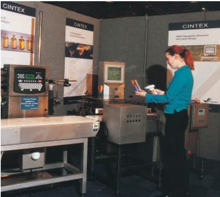
Full function checkweigher: Cintex Eclipse CS4000 (right) can be set up by scanning in the product bar code. It can then set up other line equipment such as ink jet printers (left) and metal detectors
