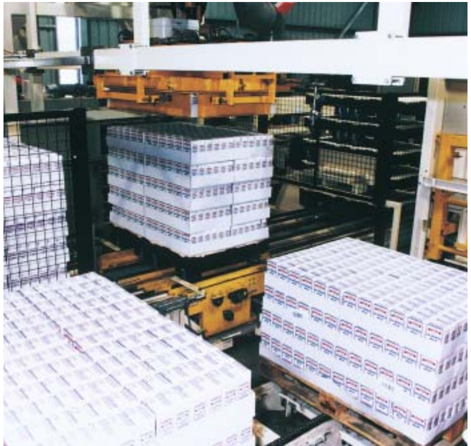
Dolly loading: Express Dairies at Credenon is using this system from Dunn Group to transfer Tetra Briks
