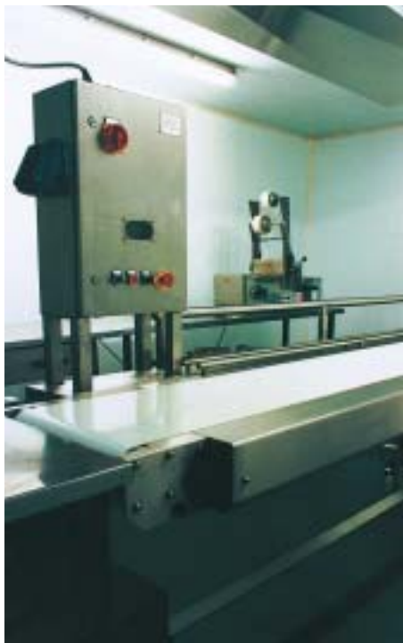
Easy belt change: Rutland cantilever design
