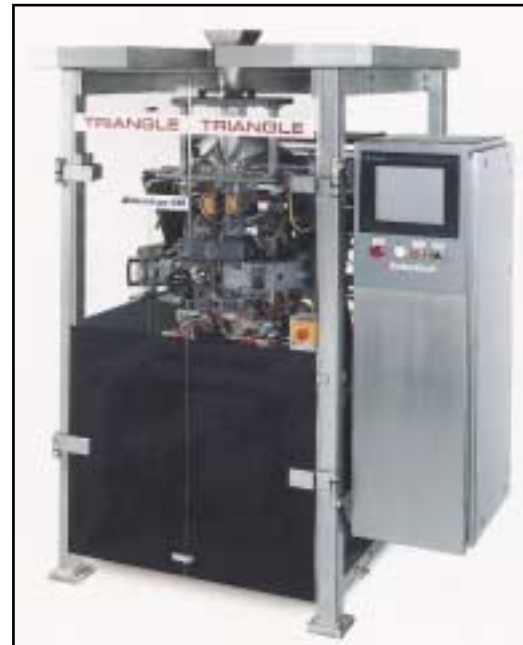
Advantage bagger: Features include interchangeable slide-in lightweight forming tubes
