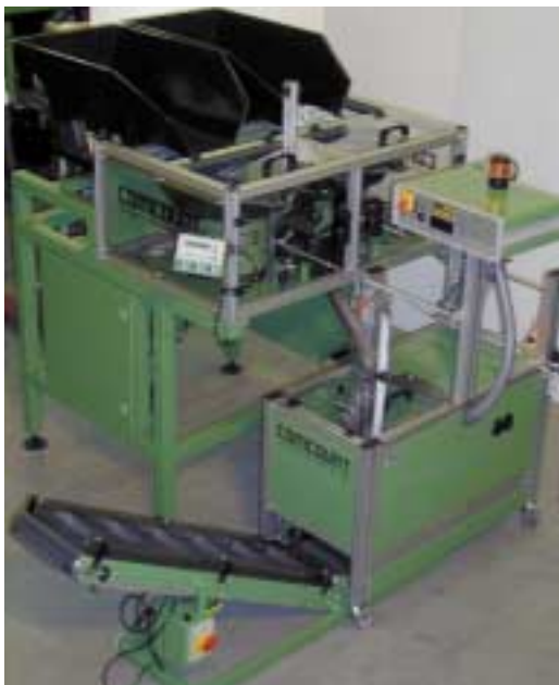
Kit packing: Twin bowl feeders and Willi W18 bagger combination from Comcount
